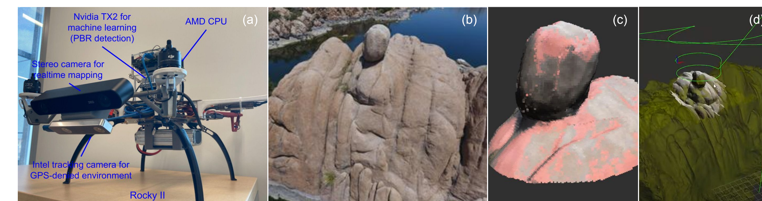
Figure 11: (a) Hexrotor with companion computers and stereo cameras found and mapped a (c) PBR at (b) Granite Dells, Prescott, Arizona. The search and mapping path is shown in Figure 11(d).
