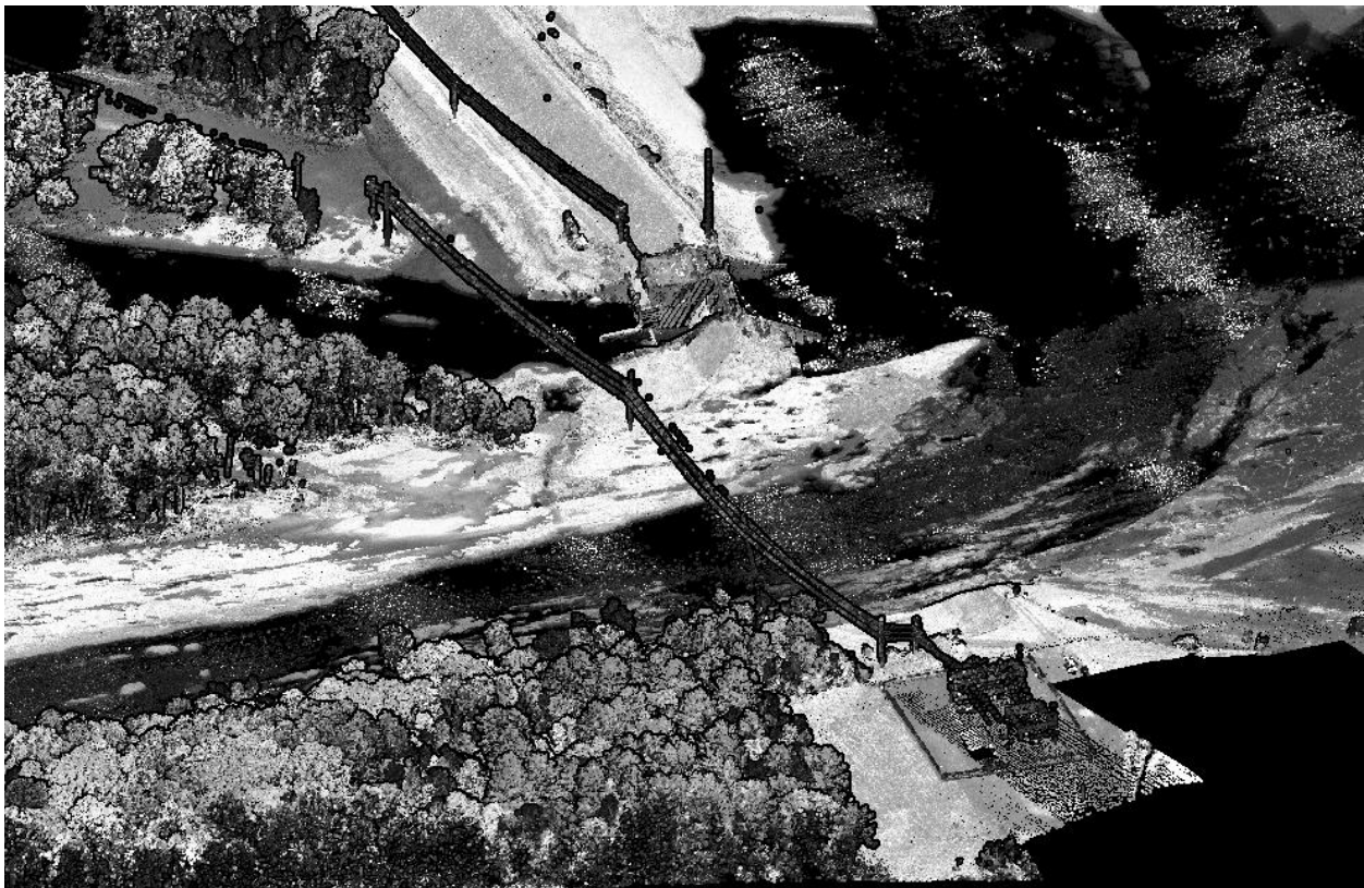
Figure 1: Oblique view of a point cloud collected by drone-based lidar showing a dam break three weeks post-failure. The dam used to run parallel to the power lines, and flow is now toward the bottom-left, having removed a wide swath of trees as escaping floodwaters formed a new channel.
