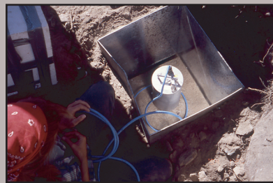
▲ Seismometers are installed in a sheltered location with good coupling to the ground
