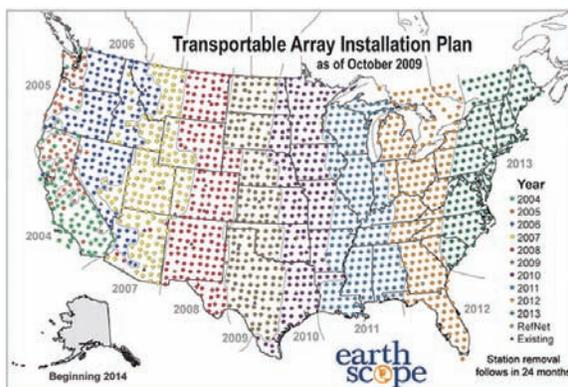
ters apart (Figure 1). During the course of the EarthScope Project, seismometers will have occupied almost 2000 sites as the array steps across the contiguous 48 states and Alaska. These seismometers remain in one location for about 24 months before being moved to their next station. In this fashion, USArray is stepping across the U.S. recording minute vibrations of Earth's surface caused by thousands of worldwide earthquakes each year. Research seismologists are analyzing
