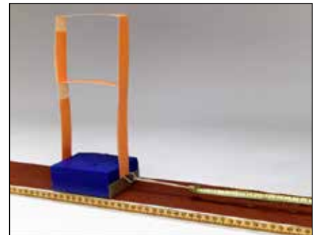
Figure 5 (right): Cardboard building attached to the Earthquake Machine.
