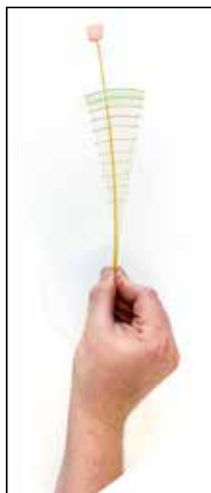
Figure 2: A piece of spaghetti with a small marshmallow will oscillate (move side to side) at its natural frequency if the tip is pulled back and then released. Image modified from Pasta Resonance .
