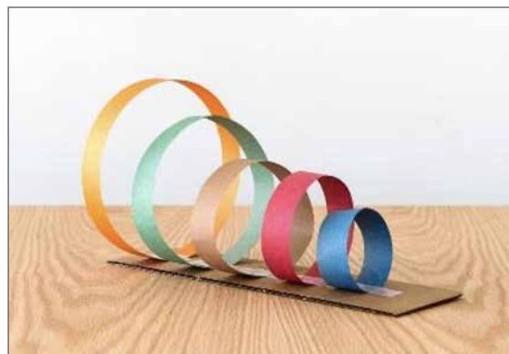
Figure 5: Resonance Rings made from construction paper. Image from the Exploratorium .
