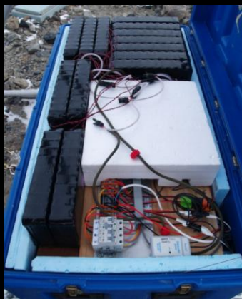
GPS w/lead acid + lithium backup
